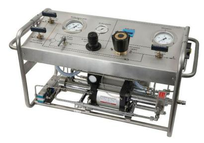
Portable Pneumatic Driven Gas Booster GBS32/SSF Air Driven Gas Booster Compressor System with Double-Acting Booster unit for Compression of Industrial Gases Argon, Helium, Hydrogen, Nitrogen and Oxygen
